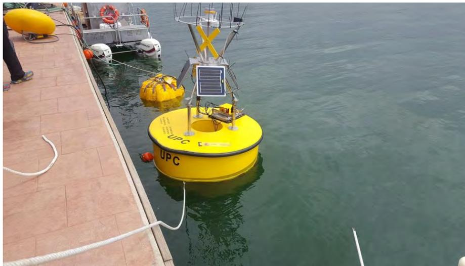
*Bloated balloon, connected to buoys-OBS and ballast*
